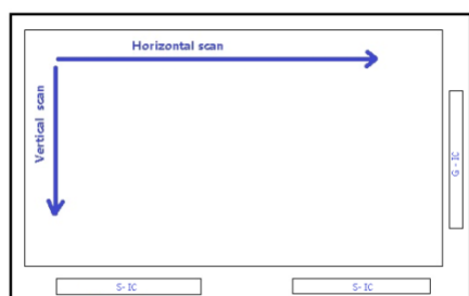
Fig. 1 Normal scan (Pin24, Reverse = Low or NC)
