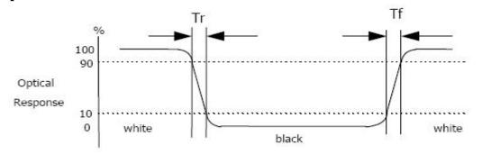
Response time is the time required for the display to transition from white to black (Rising time,  $T_r$ ) and from black to white (Falling time,  $T_f$ ) for additional information.
