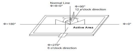
Viewing angle is the angle at which the contrast ratio is greater than 10. The angles are determined for the horizontal or x axis and the vertical or y axis with respect to the z axis which is normal to the LCD surface.
