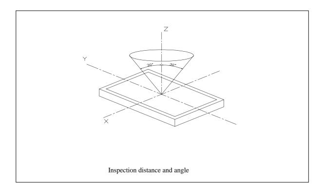
Inspection should be performed within angle  $\varphi(\phi)$  is usually 30°) from Z axis to each X and Y. Inspection distance in any direction within  $\varphi$  must be kept 30±5cm from the display surface.
