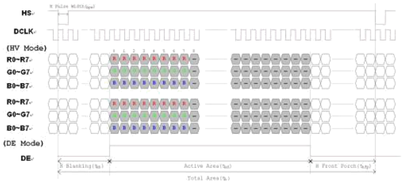
Figure 3. 1 Horizontal input timing diagram.
